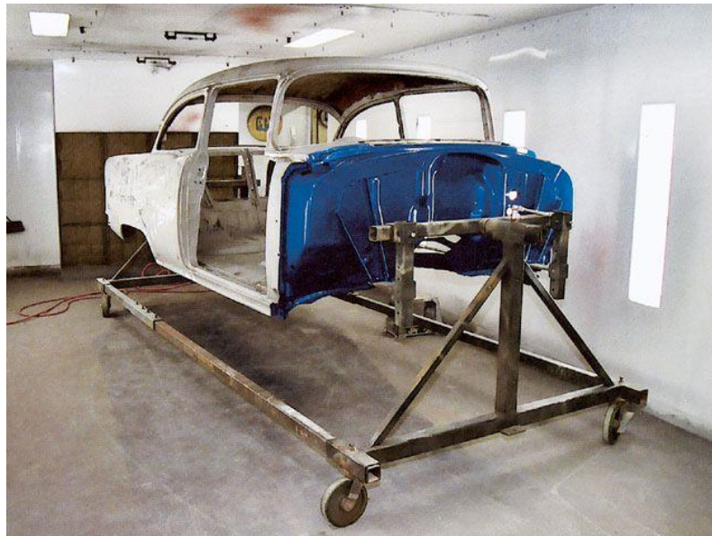
Figure 11.27. Firewall barrier protects passengers from engine fires
