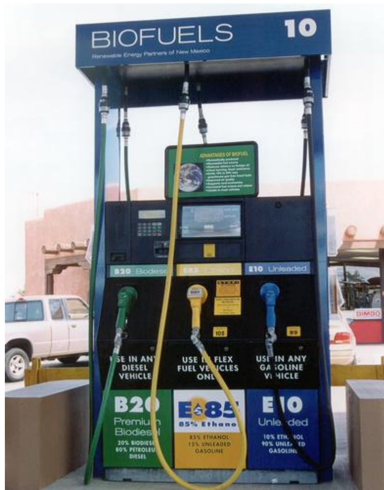
Figure 3.6 Diesel and petrol with biodiesel and ethanol blends
