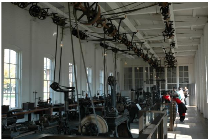
Figure 2.6. Energy from the steam engine transmitted to machines by belts and pulleys.
