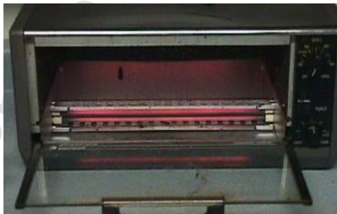
Figure 2.11. Resistor in a toaster glows red-hot.
